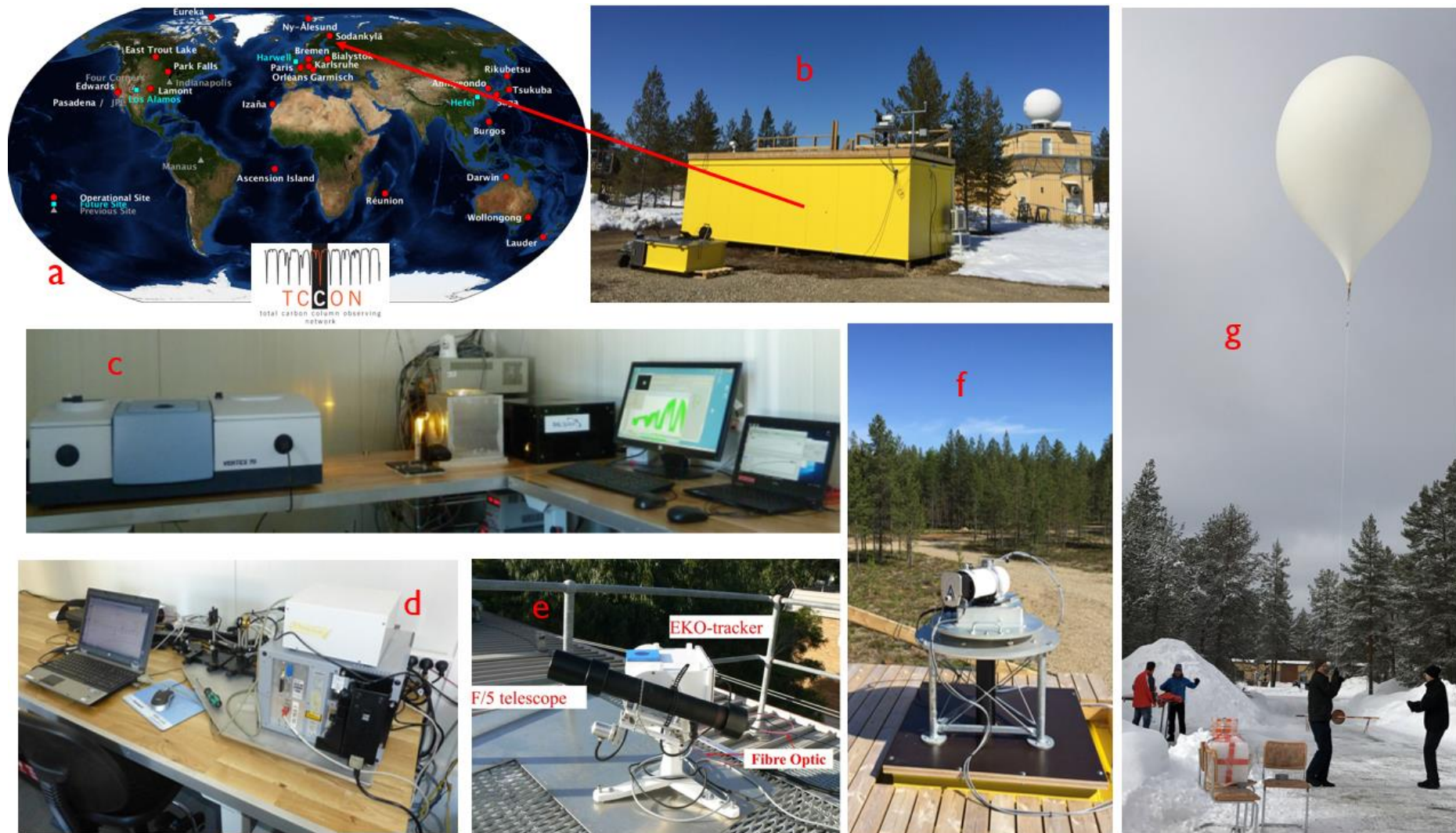
Fig. 1: (a) TCCON sites, (b) FRM4GHG container and EM27/SUN in front, (c-left) Vertex70 and (c-right) LHR, (d) IRCube, (e) suntracker for IRCube, (f) suntracker for Vertex70 and LHR, (g) Aircore launch at Sodankylä site.
