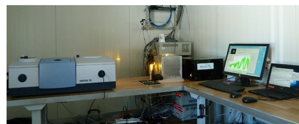
Figure 5: from left to right, LHR optical breadboard; LHR installation; H 2 O / CO 2 spectra. A second step of miniaturization has seen the system shrunk to 40x40x20 cm without loss of performance. The system has been developed to operate quasi-autonomously.
