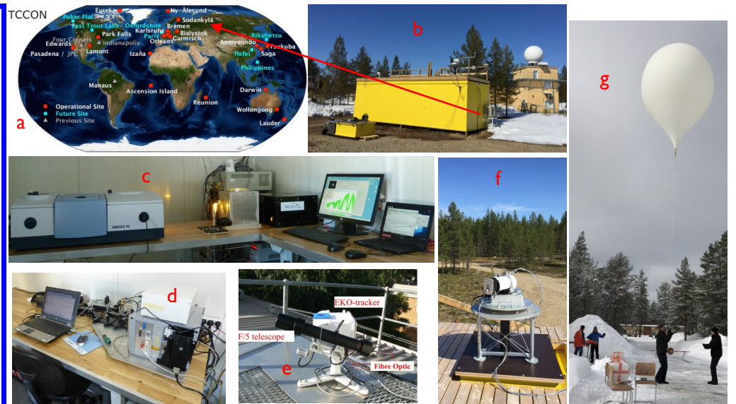
Fig. 1: (a) TCCON sites, (b) FRM4GHG container and EM27/SUN in front, (c-left) Vertex70 and (c-right) LHR, (d) IRCube, (e) suntracker for IRCube, (f) suntracker for Vertex70 and LHR, (g) Aircore launch at Sodankylä site
